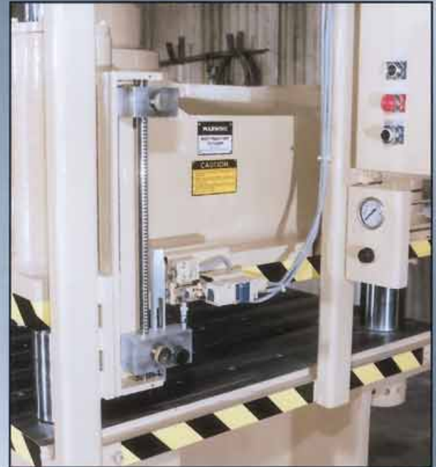
All presses come standard with a mechanical depth stop and tonnage control
