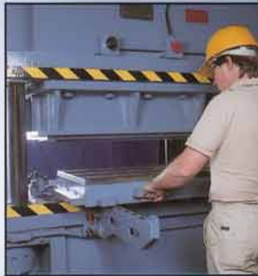
Model AP with optional bolster/die rollout arms and rubber pad holder and paint color
