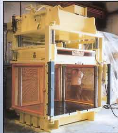
AP300 press with optional light curtains and interlocking side barriers & with special low bed height
