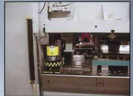
W-Technologies stroke dampers allow more punching and blanking capacity without harming hydraulic system
