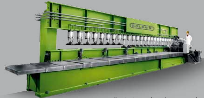
Plate chamfering machine with 12000 mm travel : length, for edges welding preparation. SAC 12000 :
