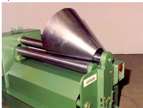
PSE 110 with tiltable top roll for cone bending.
