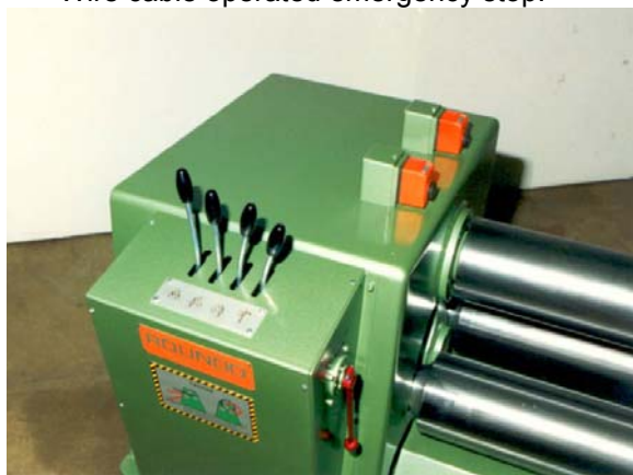
Detail of motor frame with hand levers.
